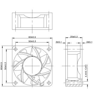
Air exhaust over struts. Rotational direction CCW looking at rotor.
